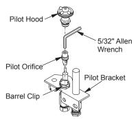
Figure 57 - Converting Pilot Orifice
